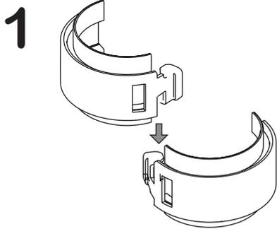
Align the two ring halves one above the other in an open position with the protruding tabs inward, then bring together until each tab sits within the slot on the other.
